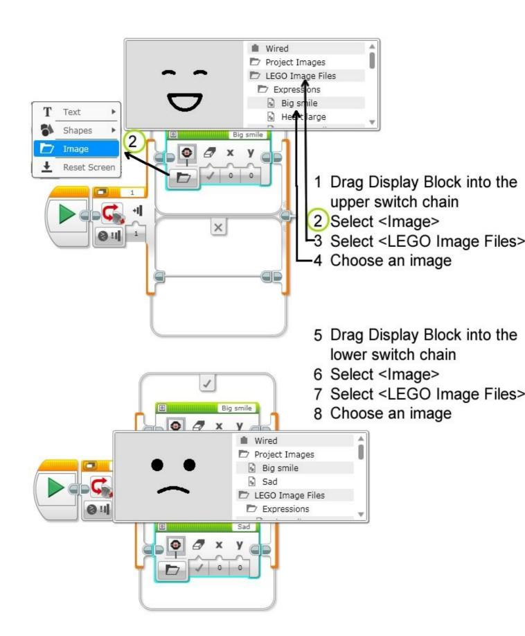
An infinite loop block needs to be added. Otherwise the switch will evaluate once.
